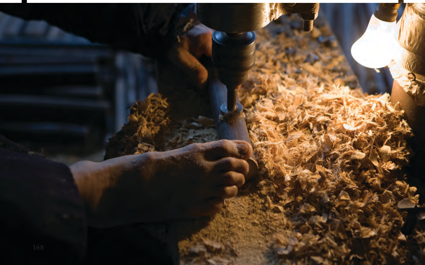
DRILLING AN EDGE MOULDING AT A FURNITURE WORKSHOP IN XUÂN LAI
