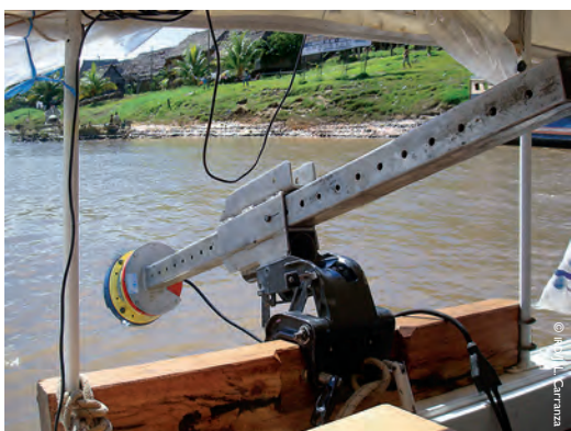
Flow measurement on Rio Marañon, Peru.
