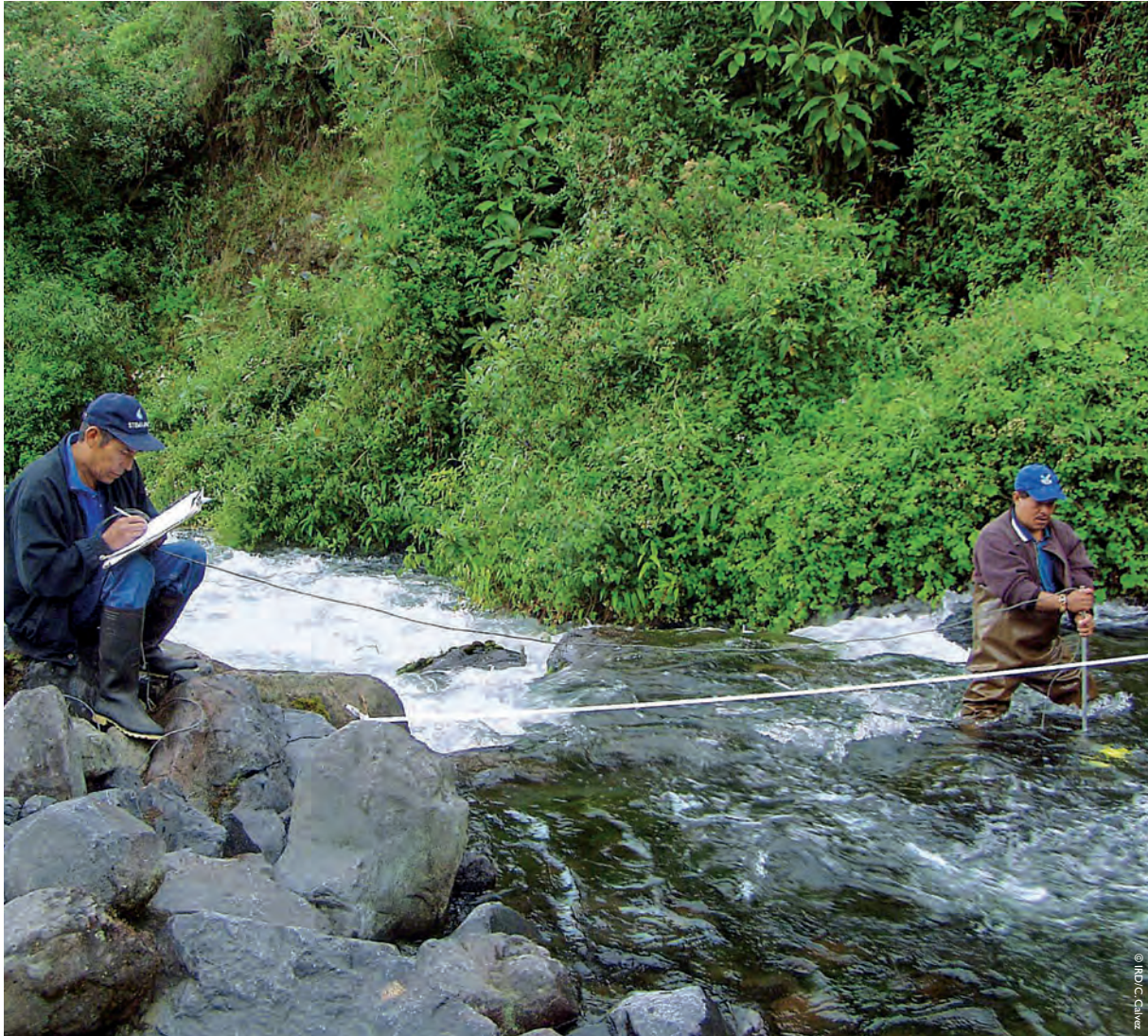
Gauging of a small stream in the Andes, Ecuador.
