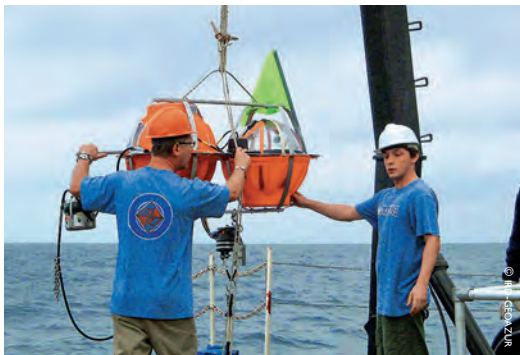
Immersion of a seismometer, Ecuador.
