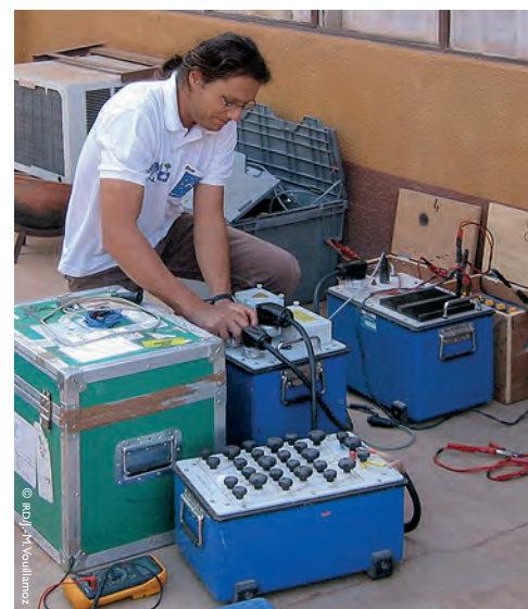
Groundwater exploration using magnetic resonance.
