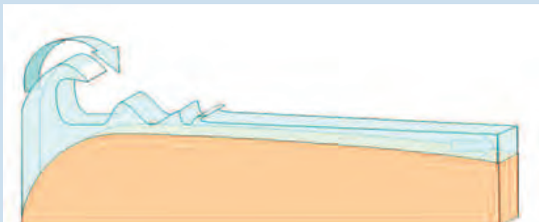
Schematic view of waves breaking over the barrier reef.
