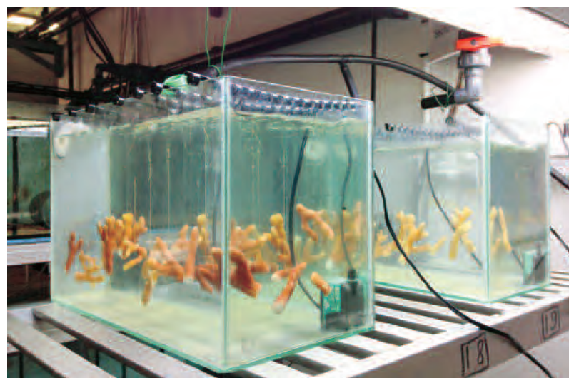
Coral colonies exposed to different cobalt concentrations and temperatures in the laboratories of the Aquarium des lagons in Nouméa. © IRD/V. Meunier
